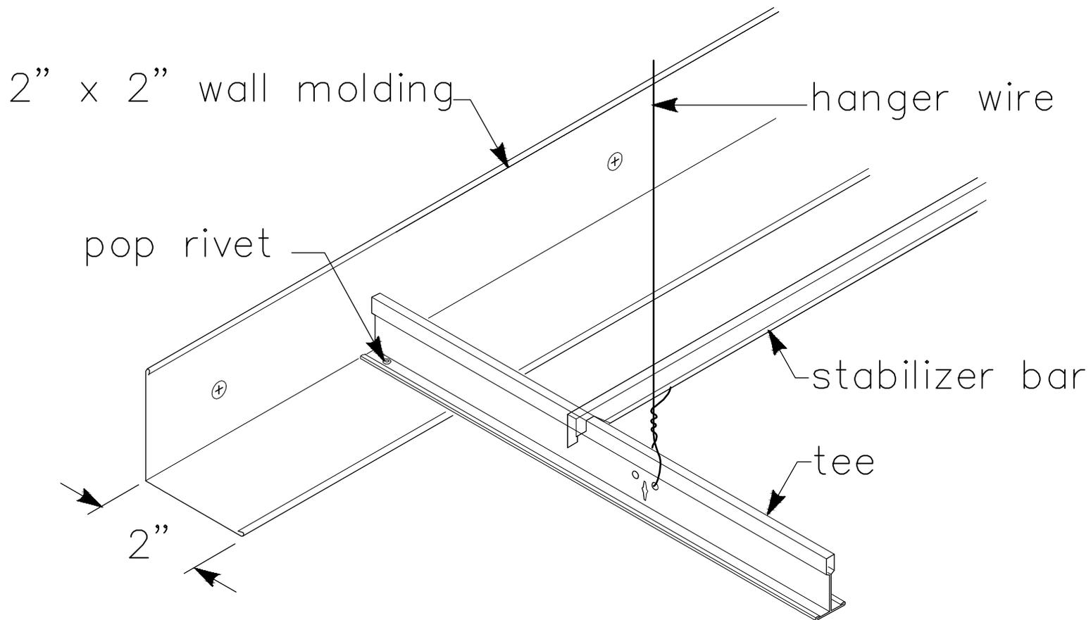
Seismic-CAT D-F-Perimeter Treatment Fixed Wall
